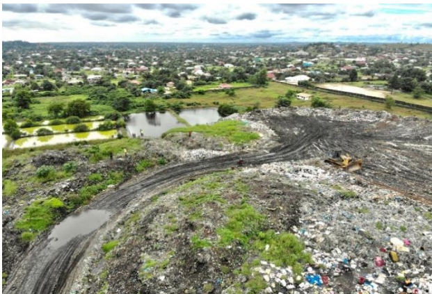
4A photo showing the access road at the top of the landfill entering the dumping space that was used for phase I drainage cleaning
