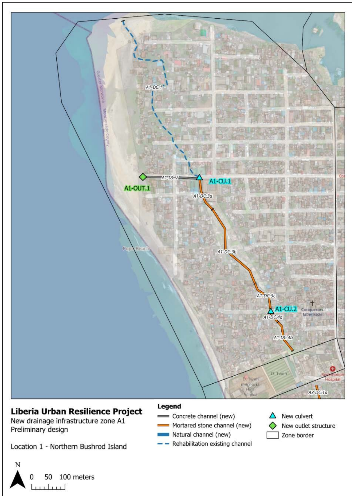
Figure 3-3 Overview of the new drainage infrastructure for Sub-location Atlantic, zone A1 (CDR International & Earthtime Inc., 2025a)
