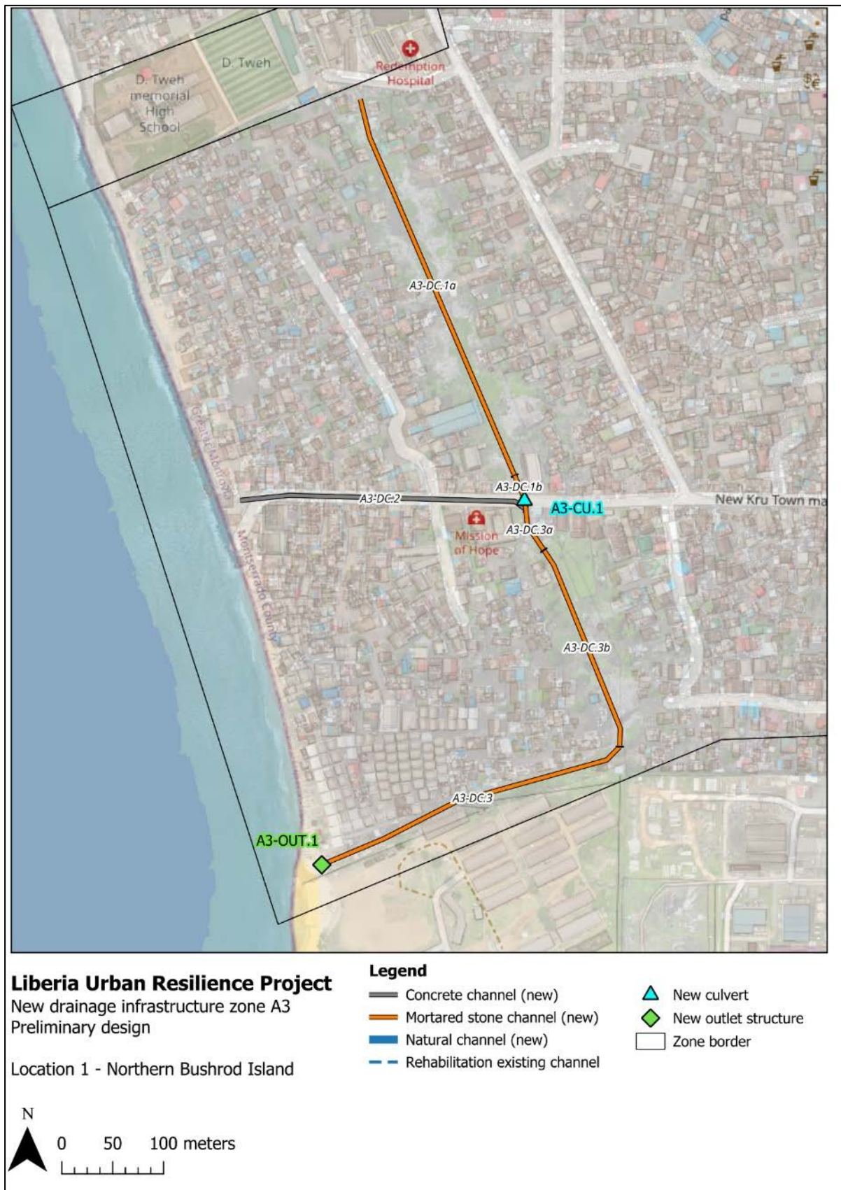
Figure 3-4 Overview of the new drainage infrastructure for Sub-location Atlantic, zone A3 (CDR International & Earthtime Inc., 2025a)
